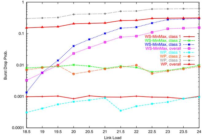
Fig. 3. Single link with  $W = 32$  wavelengths and  $P = 3$  traffic classes,  $\rho_1 = 0.2\rho, \rho_2 = 0.3\rho, \rho_3 = 0.5\rho$
