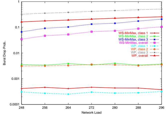
Fig. 5. NSFNet,  $W = 32$  wavelengths,  $P = 3$  traffic classes, uniform pattern,  $B_i^\ell$  obtained from (21) with  $h = D$
