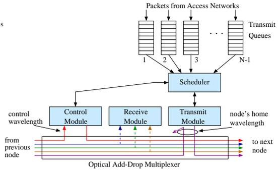
**Fig. 2.** Node architecture (delay lines not shown)
