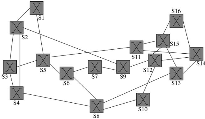
Fig. 4. 16-node topology based on the 14-node NSFNet.
