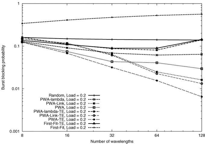
Fig. 11. Burst blocking probability, NSFNet, load = 0.2.
