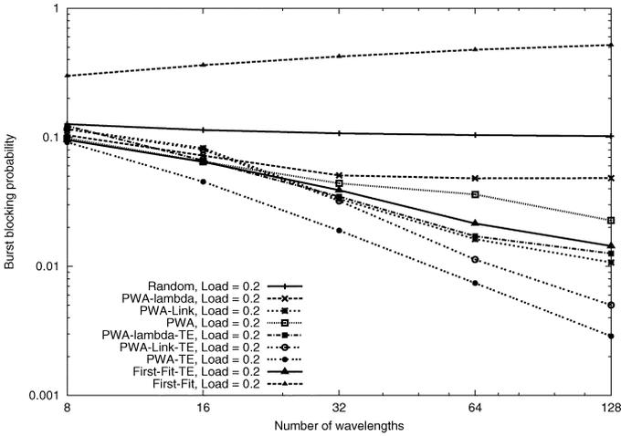
Fig. 10. Burst blocking probability, 4 x 4 torus network, load = 0.2.
