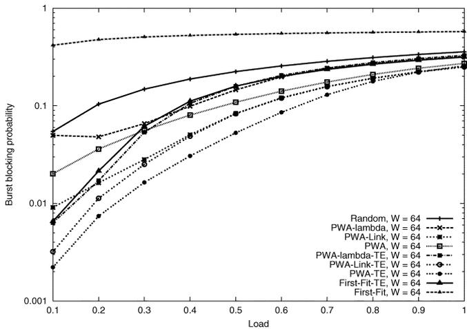
Fig. 7. Burst drop probability  $4 \times 4$  torus network, moderate and high load.
