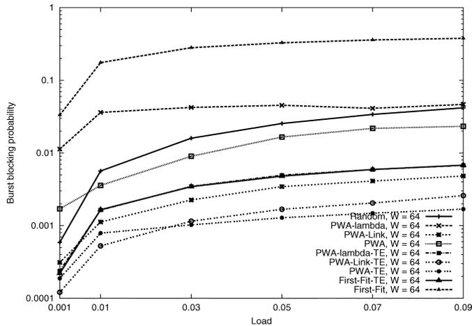
Fig. 14. Burst blocking probability,  $4 \times 4$  torus network, non-Poisson traffic, low load,  $W = 64$ .
