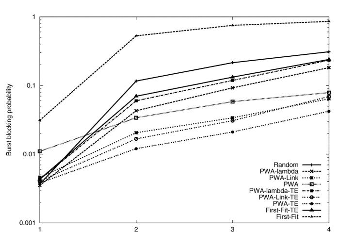
Fig. 13. Burst blocking probability, NSF network, load = 0.2,  $W = 64$ .
