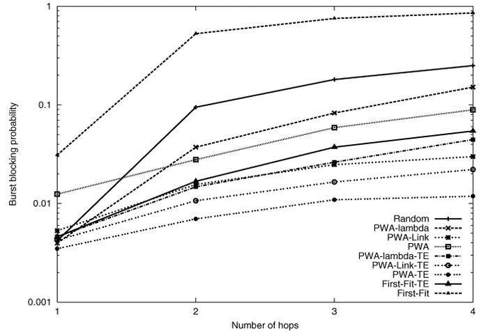
Fig. 12. Burst blocking probability, 4 x 4 torus network, load = 0.2,  $W = 64$ .
