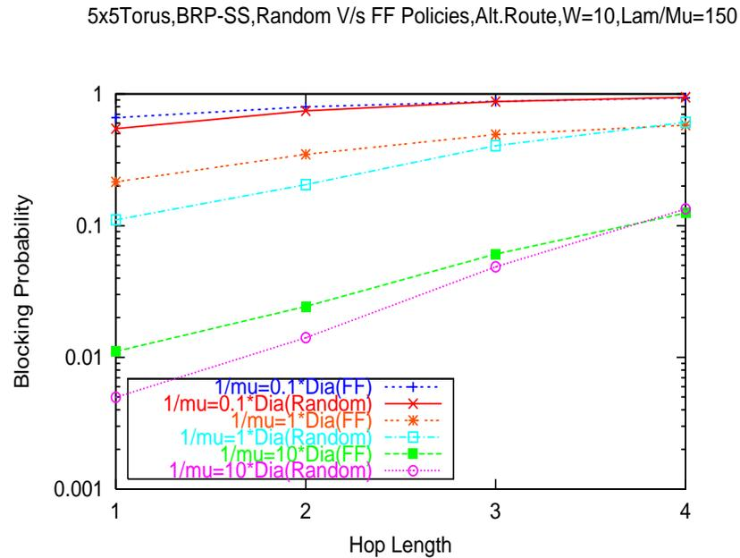
Figure 5.10: Compare Random Versus First-Fit Assignment Policy; BRP Scheme;  $5 \times 5$ -torus; Alternate Routing; Traffic load ( $\lambda/\mu$ ) = 0.25 per (S,D) pair
