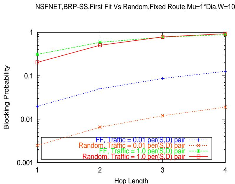
Figure 5.14: Compare Random Versus First-Fit Assignment Policy; BRP Scheme; NSFNET; Fixed Routing; Different Traffic Loads;  $1/\mu = 1 \cdot \text{Diameter}$
