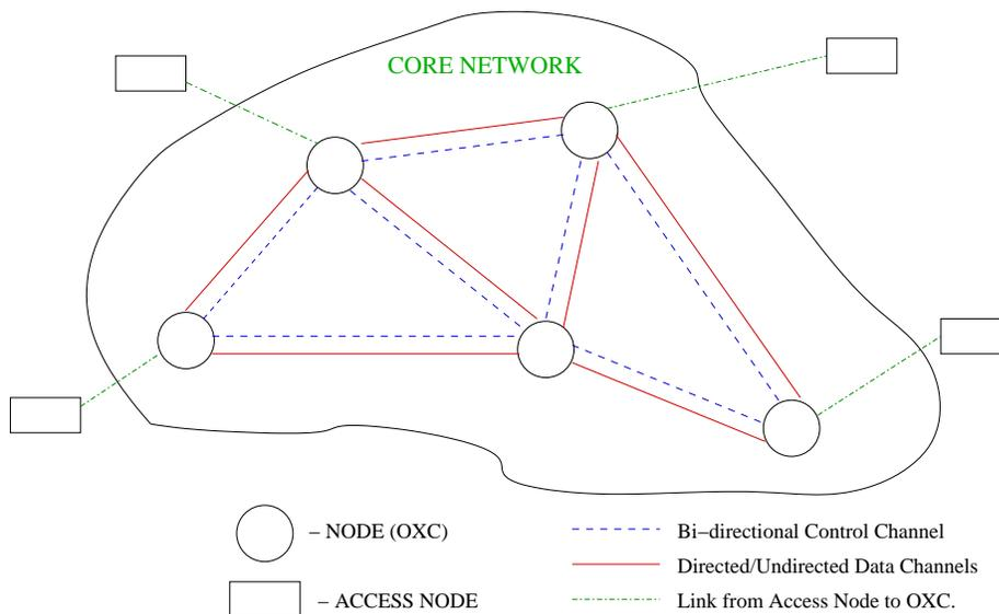
Figure 2.6: Wavelength Routed Network [19]
