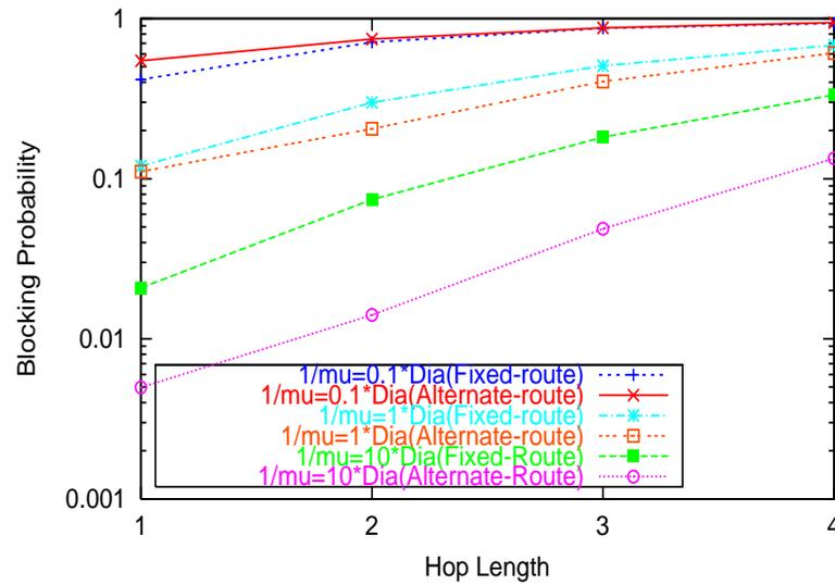
Figure 5.16: Compare Fixed (Static) Versus Alternate Routing Schemes for BRP scheme with Random policy; Traffic load ( $\lambda/\mu$ ) = 0.25 per (S,D) pair
