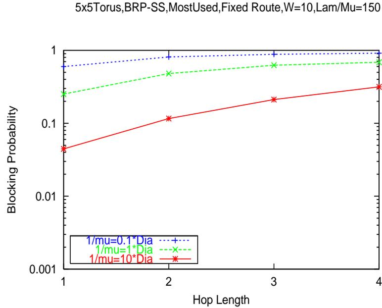
Figure 5.8: Blocking Probability increases as average holding time ( $1/\mu$ ) decreases relative to the signaling delays; Traffic load ( $\lambda/\mu$ ) = 0.25 per (S,D) pair
