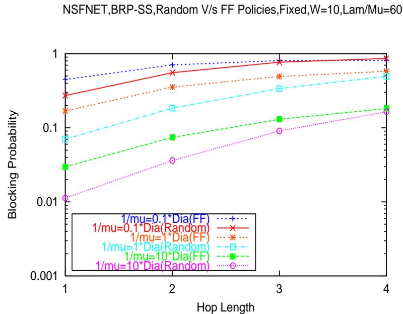
Figure 5.11: Compare Random Versus First-Fit Assignment Policy; BRP Scheme; NSFNET; Fixed Routing; Traffic load ( $\lambda/\mu$ ) = 0.25 per (S,D) pair
