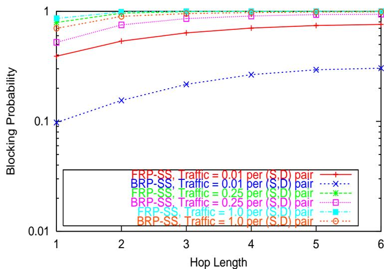
Figure 5.23: Compare BRP-SS scheme with FRP-SS scheme; 12-node Ring; Alternate Route; First-fit policy;  $1/\mu = 0.1*\text{Diameter}$
