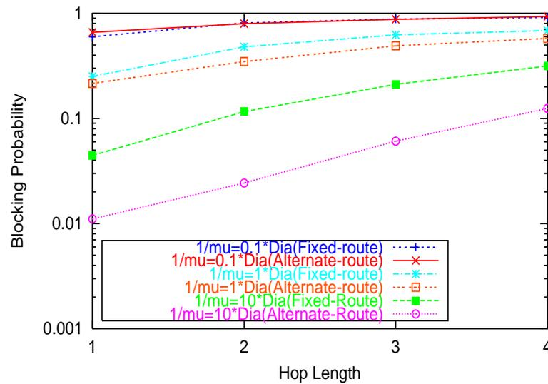
Figure 5.17: Compare Fixed (Static) Versus Alternate Routing Schemes for BRP scheme with Most-Used policy; Traffic load ( $\lambda/\mu$ ) = 0.25 per (S,D) pair
