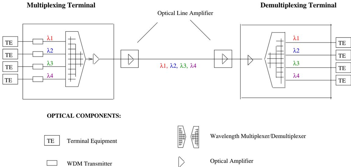
Figure 2.1: Point to Point WDM Systems [19]
