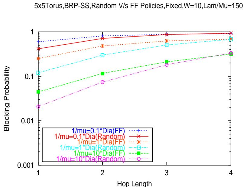
Figure 5.9: Compare Random Versus First-Fit Assignment Policy; BRP Scheme;  $5 \times 5$ -torus; Fixed Routing; Traffic load  $(\lambda/\mu) = 0.25$  per (S,D) pair
