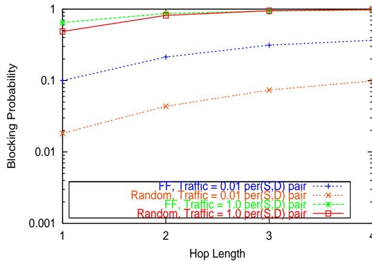
Figure 5.13: Compare Random Versus First-Fit Assignment Policy; BRP Scheme; NSFNET; Fixed Routing; Different Traffic Loads;  $1/\mu = 0.1 \cdot \text{Diameter}$
