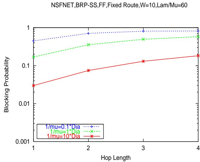
Figure 5.4: Blocking Probability increases as average holding time ( $1/\mu$ ) decreases relative to the signaling delays; FF = First Fit, Traffic load ( $\lambda/\mu$ ) = 0.25 per (S,D) pair
