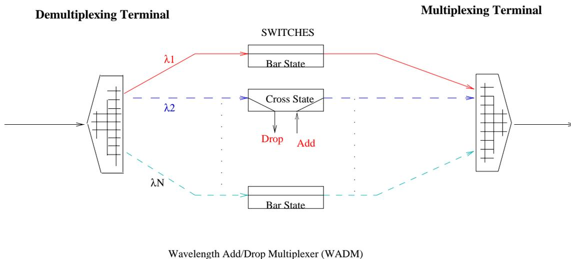
Figure 2.2: Wavelength Add/Drop Multiplexer (WADM) [19]
