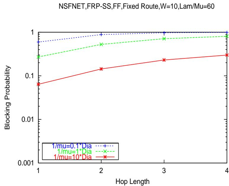
Figure 5.5: Blocking Probability increases as average holding time ( $1/\mu$ ) decreases relative to the signaling delays; FF = First Fit, Traffic load ( $\lambda/\mu$ ) = 0.25 per (S,D) pair
