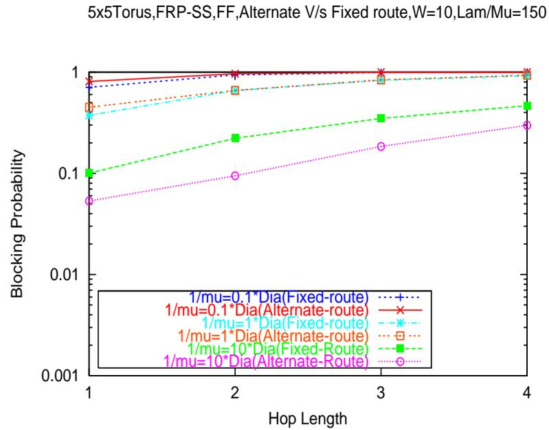
Figure 5.18: Compare Fixed (Static) Versus Alternate Routing Schemes for FRP scheme with First-fit policy; Traffic load  $(\lambda/\mu) = 0.25$  per (S,D) pair
