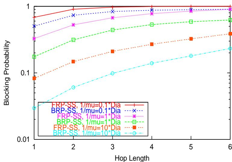
Figure 5.22: Compare BRP-SS scheme with FRP-SS scheme; 12-node Ring; Fixed Route; First-fit policy; Traffic load  $(\lambda/\mu) = 0.25$  per (S,D) pair
