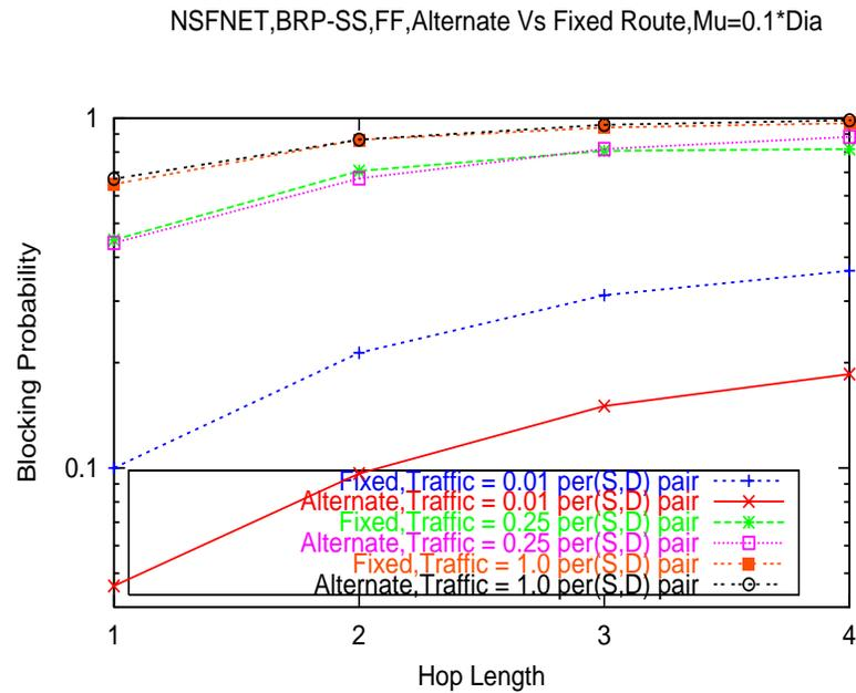
Figure 5.19: Compare Fixed (Static) Versus Alternate Routing Schemes for BRP scheme with First-fit policy;  $1/\mu = 0.1 \cdot \text{Diameter}$
