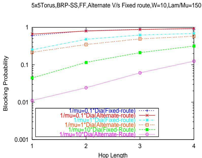
Figure 5.15: Compare Fixed (Static) Versus Alternate Routing Schemes for BRP scheme with First-Fit policy; Traffic load  $(\lambda/\mu) = 0.25$  per (S,D) pair
