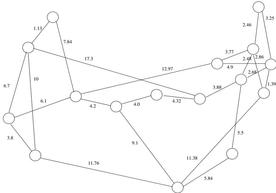
Figure 5.3: NSFNET Topology; Approximate propagation delays are given based on distance between cities
