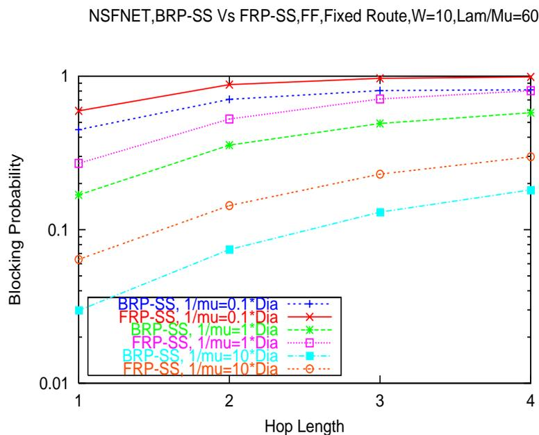
Figure 5.21: Compare BRP-SS scheme with FRP-SS scheme; NSFNET; First-fit policy; Fixed Routing; Traffic load ( $\lambda/\mu$ ) = 0.25 per (S,D) pair
