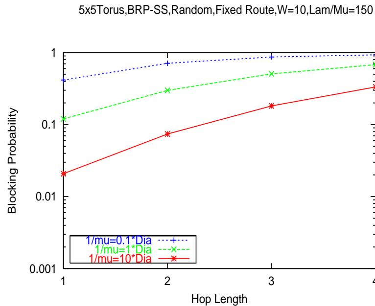
Figure 5.7: Blocking Probability increases as average holding time ( $1/\mu$ ) decreases relative to the signaling delays; Traffic load ( $\lambda/\mu$ ) = 0.25 per (S,D) pair
