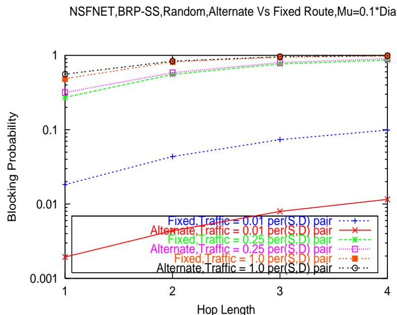
Figure 5.20: Compare Fixed (Static) Versus Alternate Routing Schemes for BRP scheme with Random policy;  $1/\mu = 0.1 * \text{Diameter}$
