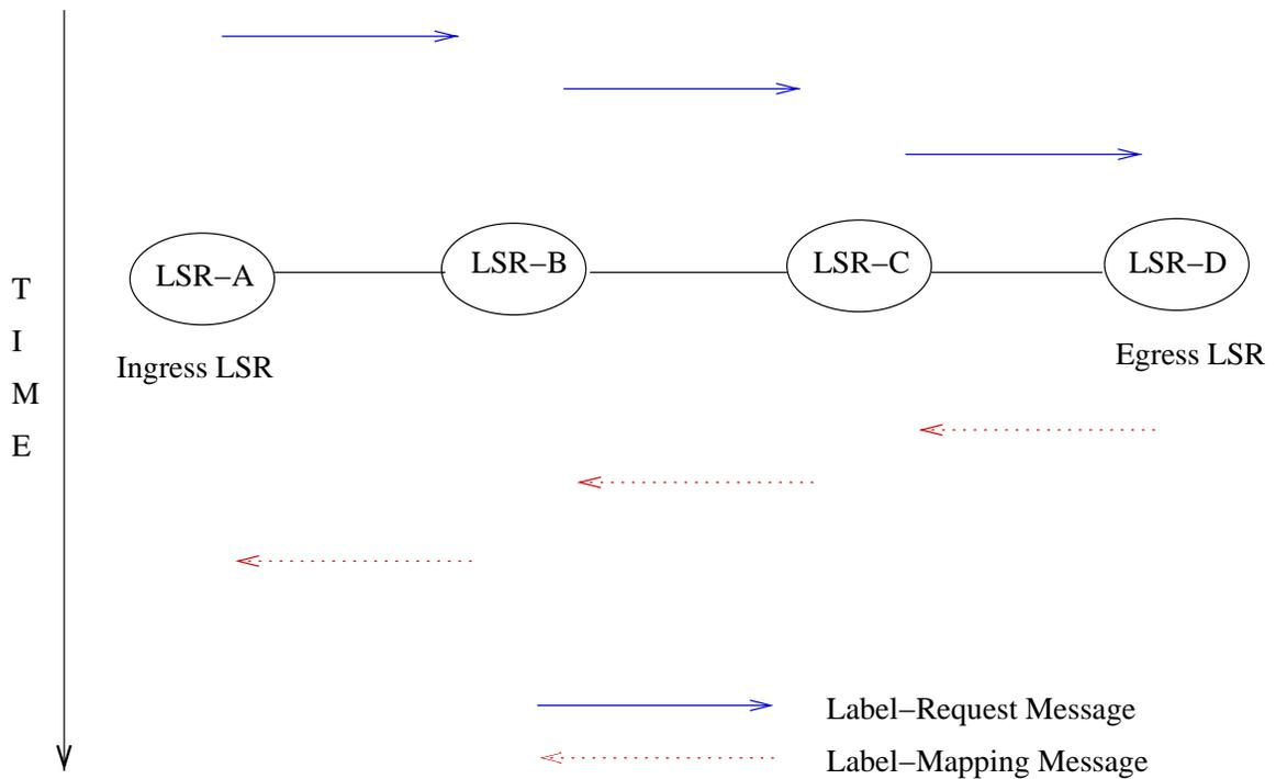
Figure 3.1: Constrained-Routed Label Switched Path - Establishment (Message exchange)
