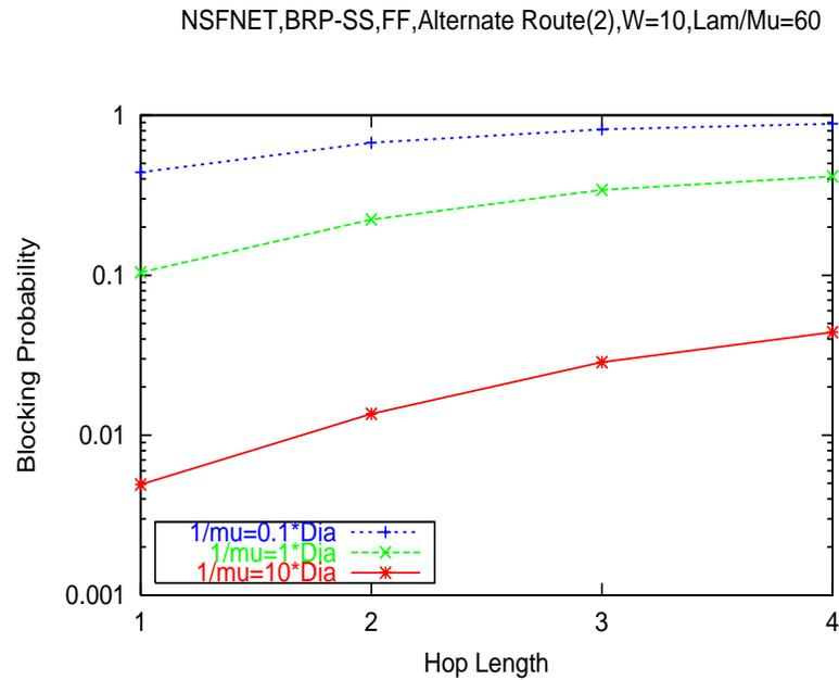
Figure 5.6: Blocking Probability increases as average holding time ( $1/\mu$ ) decreases relative to the signaling delays; FF = First Fit, Traffic load ( $\lambda/\mu$ ) = 0.25 per (S,D) pair, Alternate Route with 2 pre-computed paths
