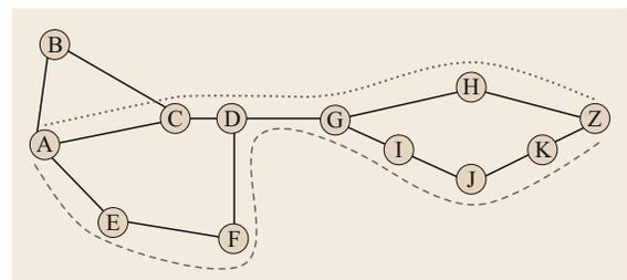
**Fig. 12.6** There is no completely disjoint pair of paths between nodes A and Z. The set of paths shown by the *dotted* and *dashed lines* represents the shortest maximally-disjoint pair of paths. The paths have nodes D and G, and the link between them, in common (© Monarch Network Architects LLC)
