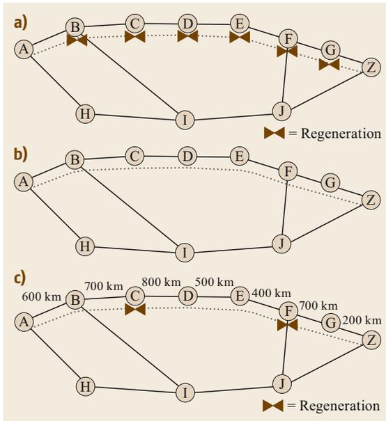
**Fig. 12.1a–c** The connection path from node A to node Z is shown by the dotted line. (a) In an O-E-O network, regeneration occurs at each node along the path of the connection. (b) In a true all-optical network, there is no regeneration along the path. The connection remains in the optical domain from end to end. (c) With an optical reach of 2000 km and the link distances as shown, two regenerations are required for the connection. (© Monarch Network Architects LLC)
