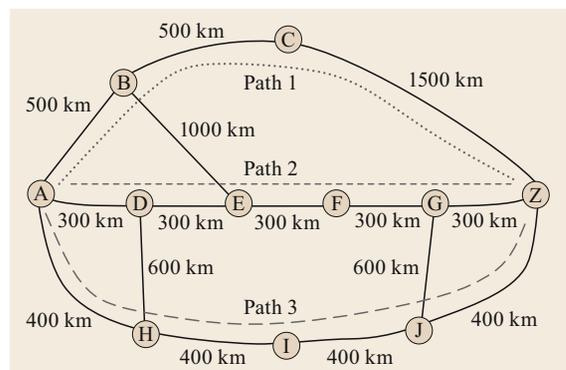
**Fig. 12.3** Assume that this is an all-optical network with an optical reach of 2000 km. Path 1, A–B–C–Z, has the fewest hops but requires one regeneration. Path 2, A–D–E–F–G–Z, and Path 3, A–H–I–J–Z, require no regeneration. Of these two lowest-cost paths, Path 3 is preferred because it has fewer hops (© Monarch Network Architects LLC)
