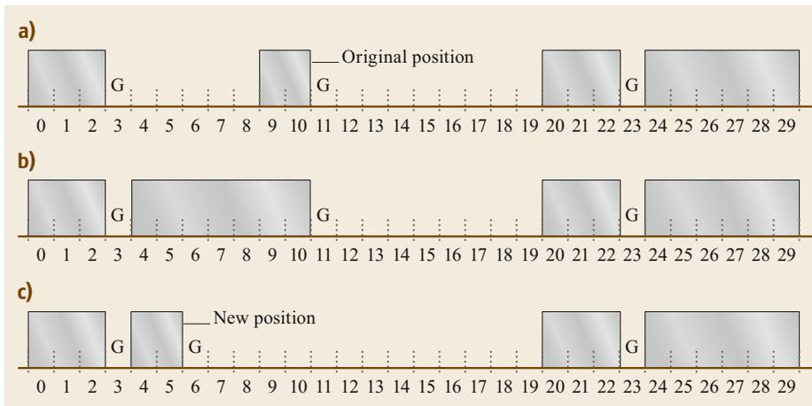
**Fig. 12.20a–c** Push–pull defragmentation. **(a)** The original spectral partitioning. Assume that it is desired to shift the optical channel on slots 9 and 10 to slots 4 and 5 on that same link. **(b)** In the first phase, the channel is extended to encompass the original slots, the new slots, and any slots in between. **(c)** In the second phase, the channel is contracted to encompass just the new slots, 4 and 5
