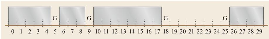
**Fig. 12.17** In this depiction, the spectrum is divided into 30 spectral slots. Four optical channels are assigned on the fiber, as indicated by the *shaded boxes*; *G* indicates a guardband slot (© Monarch Network Architects LLC)
