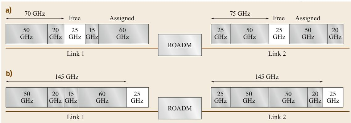
**Fig. 12.19a,b** Assume that a new optical channel requiring 25 GHz of spectrum needs to be routed across links 1 and 2. **(a)** Both links have an available 25 GHz gap; however, the gaps are not aligned. The optical channel cannot be routed all-optically through the ROADM, but instead would be regenerated to accomplish spectrum conversion. **(b)** After defragmentation, the assigned spectrum forms a contiguous block, leaving the available spectrum aligned (© Monarch Network Architects LLC)
