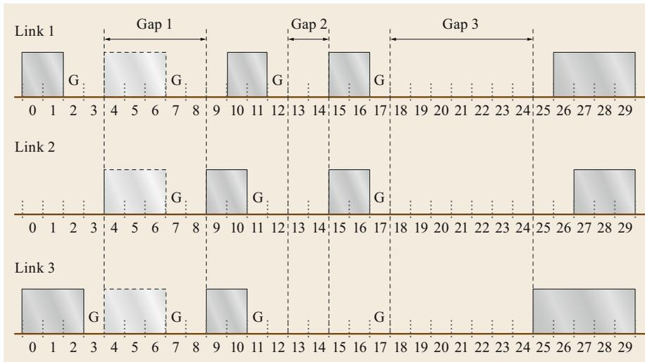
**Fig. 12.18** A new optical channel, requiring a total of four slots, is routed all-optically on three links. The *solid shaded slots* indicate spectrum that has previously been assigned. Of the three existing gaps, the best-fitting one is gap 1. The new optical channel, represented by the *hatched slots*, is shown assigned to this gap. This strands bandwidth on link 1 (slot 3) and on links 2 and 3 (slot 8) (© Monarch Network Architects LLC)
