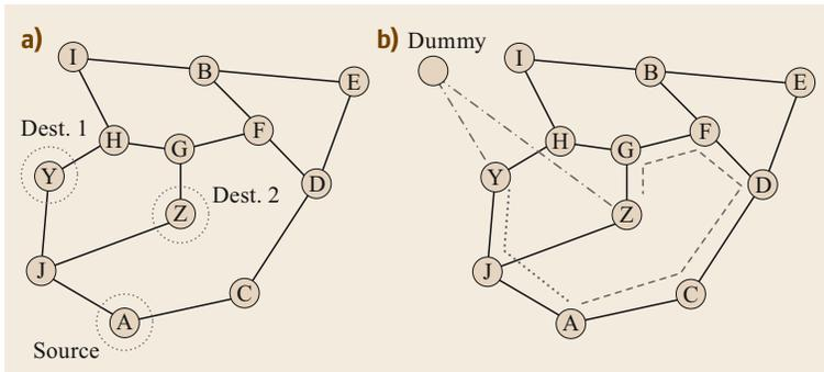
**Fig. 12.7** (a) A disjoint path is desired between one source (node A) and two destinations (nodes Y and Z). (b) A dummy node is added to the topology and connected to the two destinations via links that are assigned a metric of zero. A shortest-disjoint-paths algorithm is run between node A and the dummy node to implicitly generate the desired disjoint paths, as shown by the dotted line and the dashed line (© Monarch Network Architects LLC)
