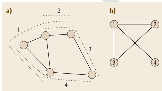
**Fig. 12.14** (a) Four all-optical segments, each one numbered, are routed as indicated by the *dotted lines*. It is assumed that there is one fiber-pair on each link. (b) The resulting conflict graph, where each node represents one of the all-optical segments. A link exists between two nodes if the corresponding all-optical segments are routed on the same fiber on any link in the original graph
