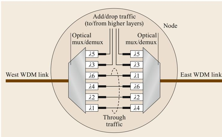
**Fig. 12.12** A representative node in an O-E-O network. Wavelengths can be assigned independently to the connections on each link as long as each wavelength assigned on a fiber is unique. The lower-most connection is carried on  $\lambda_1$  on the West link and carried on  $\lambda_4$  on the East link (© Monarch Network Architects LLC)
