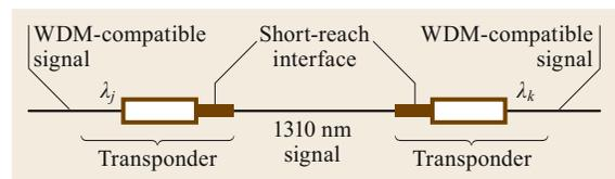
**Fig. 12.11** Regeneration through the use of back-to-back transponders. The WDM-compatible signals associated with the two transponders,  $\lambda_j$  and  $\lambda_k$ , do not have to be the same, thereby enabling wavelength conversion (© Monarch Network Architects LLC)
