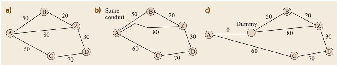
**Fig. 12.8** (a) In the link-level view of the topology, links AB and AZ appear to be disjoint. (b) In the fiber-level view, these two links lie in the same conduit exiting node A and are, thus, not fully diverse. A single cut to this section of conduit can cause both links to fail. (c) Graph transformation to account for the SRLG extending from node A (© Monarch Network Architects LLC)
