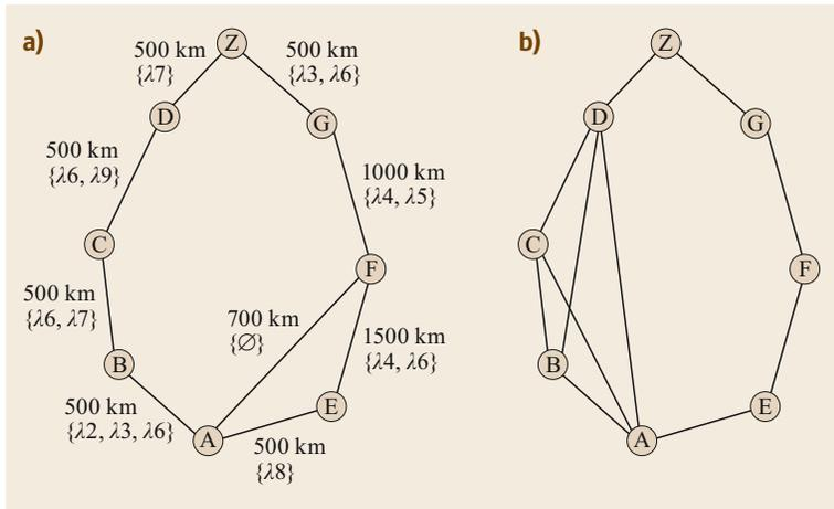
**Fig. 12.15** (a) The true network topology, where it is assumed that the optical reach is 2000 km. The wavelengths listed next to each link are the wavelengths that are assumed to be free on the link. (b) The reachability graph, where a link is added between a node pair if there is a regeneration-free path between the nodes with at least one available wavelength along the path (© Monarch Network Architects LLC)
