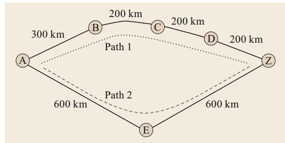
**Fig. 12.2** Path 1, A–B–C–D–Z, is the shortest-distance path between nodes A and Z, but Path 2, A–E–Z, is the fewest-hops path. In an O-E-O network, where the signal is regenerated at every intermediate node, Path 2 is typically the lower-cost path (© Monarch Network Architects LLC)
