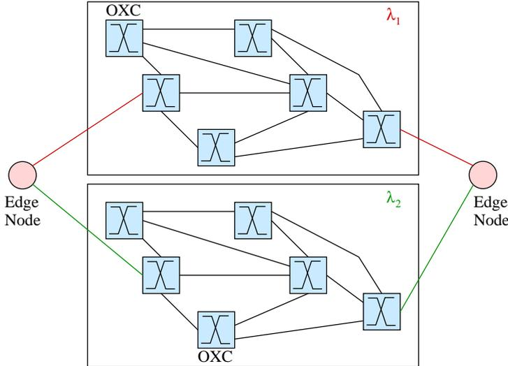
Figure 3: The RWA problem with two wavelengths per fiber
