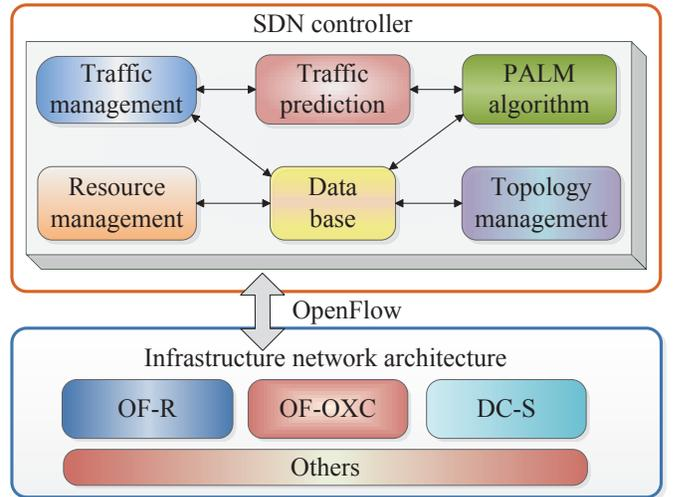
Fig. 2. The functional modules of controller in software defined EONs for DC application
