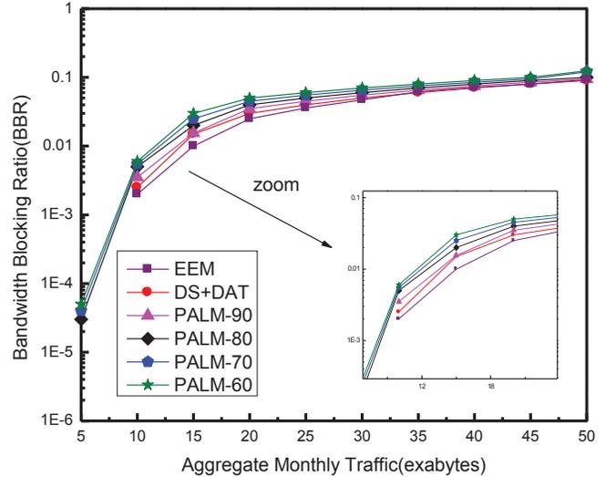
Fig. 8. Algorithm comparison with respect to BBR
