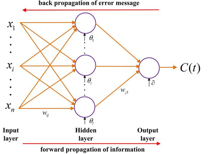
Fig. 3. Configuration of a 3-layer BP network model
