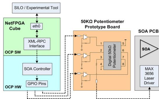
Fig. 2. NetFPGA-based OCP enables cross-layer communication between the optical layer and higher network layers.
